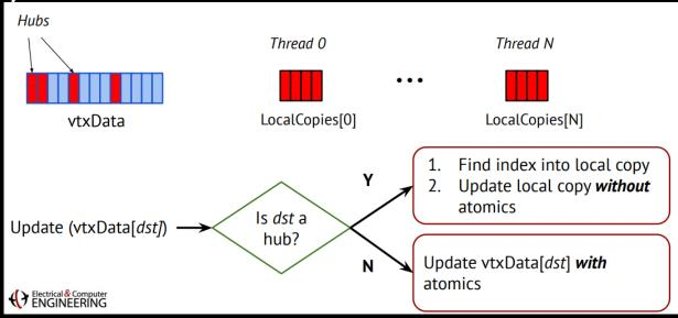
Expensive overheads: lookup in a an extra data structure when visiting each vertex to figure out if it's a "hub" to index into the tread-local copies.
