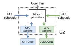
Fig. 1. G2 adds a new GPU backend to GraphIt that produces CUDA code from the same GraphIt algorithm language and a scheduling language tailored for GPU optimizations.
