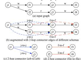
**Fig. 3:** Construction of different 2-hop connector graph views over a heterogeneous network (namely, a data lineage graph) with two vertex types (N = 2) and two edge types (M = 2).
