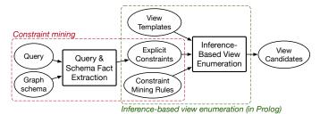
Fig. 4: Constraint-based view enumeration in KASKADE.
