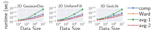
Figure 8: Runtimes (seconds) of our algorithm “PC” on three data sets of varying sizes using 48 cores with two-way hyper-threading. The “Ward” and “avg-2” lines overlapped because they have similar runtimes. The results show that the scalability is very similar across datasets.
